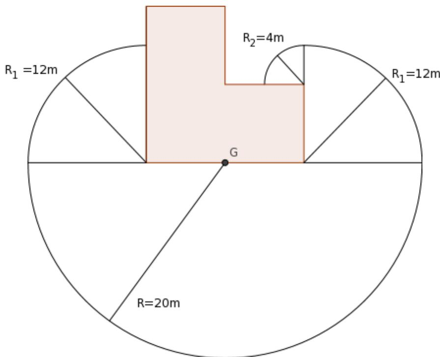
$$Area = \pi \frac{R^2}{2} + \left( \pi \frac{R_1^2}{4} \right) 2 + \pi \frac{R_2^2}{4} = 3.14 \left( \frac{400}{2} + \frac{144}{2} + \frac{16}{4} \right) = 866.64$$
